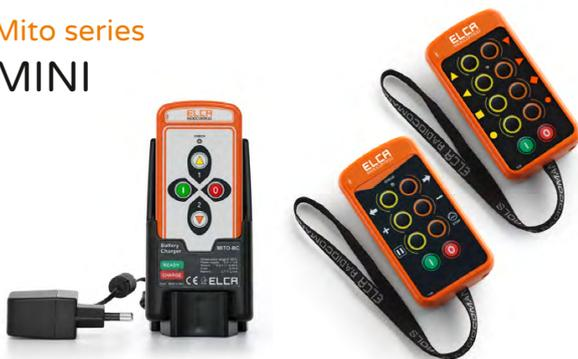
MINI is a compact radiocontrol to control remotely a wide range of industrial automation applications. Versions from 4 to 10 single step buttons Control panel and function modes are programmable, IP67, floatable. Bi-directional technology LBT with automatic frequency change, while working a LED "check" to confirm active radio connection with receiver. Internal Lithium battery (up to 50 hours). Configurations with multiple transmitters/receivers.
