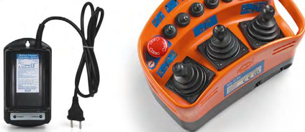
Joystick radiocontrol SFERA has the same characteristics of PUNTO model even if slightly bigger to host 3 on/off joysticks, single or double axis (series Genio) or 3 proportional joysticks or 6 single axis (series E1), 5 toggle switch, removable activation key and Stop push-button. Transmitter can be adapted to customer needs. Powered by interchangeable battery with dedicated charger.
