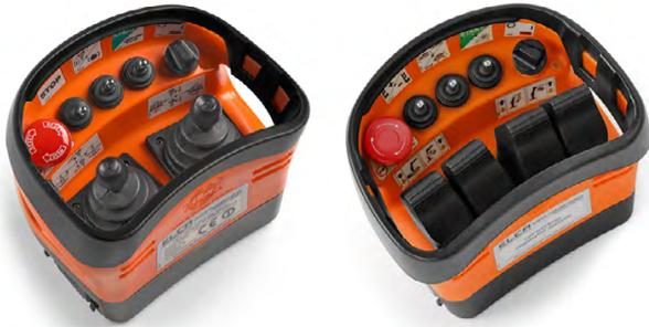
PUNTO is a compact joystick radiocontrol. Standard configurations with 2 on/off joysticks, single or double axis (series Genio) or 2 proportional joystick or 4 mono axis (series E1), 3 toggle switches, removable activation key and Stop push-button. Transmitter is customizable according to specifications supplied by the customer. Powered by interchangeable battery with dedicated charger.
