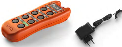
Evo is Elca's standard handheld radiocontrol for machines and industrial lifting and handling. It consists of 6 double step push-buttons, 1 programmable function button, Start with programmable code activation key and Stop. Auto switch off, IP65, internal Lithium battery (up to 20 hours) with power supply ELCA-CLIP. Optional "Master-Slave" and "multi-transmitter".
