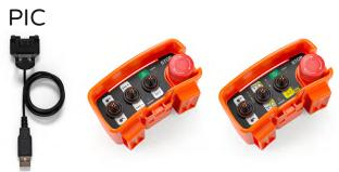
PIC is a compact waistbelt radiocontrol, small and lightweight, robust and reliable. Designed to satisfy a vast range of applications (compatible with MITO and E1 electronics). The standard configuration consists of 3 selectors and emergency mushroomshaped stop button, allowing for 5 commands, and with a second function toggle, up to 8 commands. Interchangeable Lithium battery.
