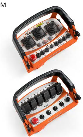
Model M transmitter is the winning choice for its flexibility and available surface. Can be fitted with single or double axis joystick and permits a wide range of layout: potentiometers, toggle switches, many kind of buttons, with up to 6 proportional outputs (8 Bravo series) and 28 on/off commands.
